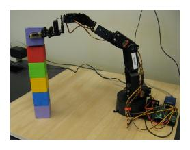
Figure 3.15 The robotic arm needs to rotate its joints in order to pick up objects or to place them correctly. Figure taken from (Deisenroth et al., 2015).
